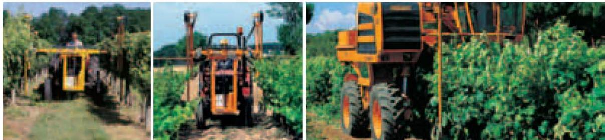
The reciprocating cutting bars cut the **branches cleanly** as would pruning shear blades.
