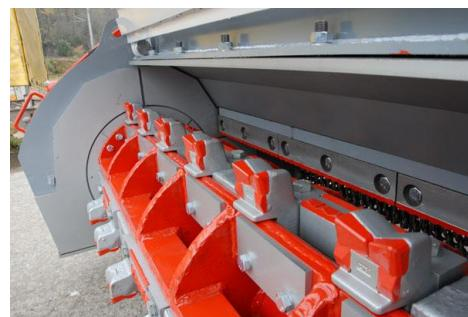
SLIKA 12 KONSTRUKCIJA ALATA PTH DROBILICE
